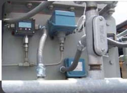
The One Series and other switches monitoring lube oil on a gear box.
